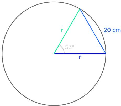
$$\begin{aligned}a^2 &= b^2 + c^2 - 2bc \cdot \cos A \\20^2 &= r^2 + r^2 - 2(r)(r) \cos 53^\circ \\400 &= 2r^2 - 2r^2(3/5) \\400(5) &= 2(5)r^2 - 6r^2 \\2000 &= 4r^2 \\500 &= r^2 \\\sqrt{500} &= 10\sqrt{5} = r\end{aligned}$$
